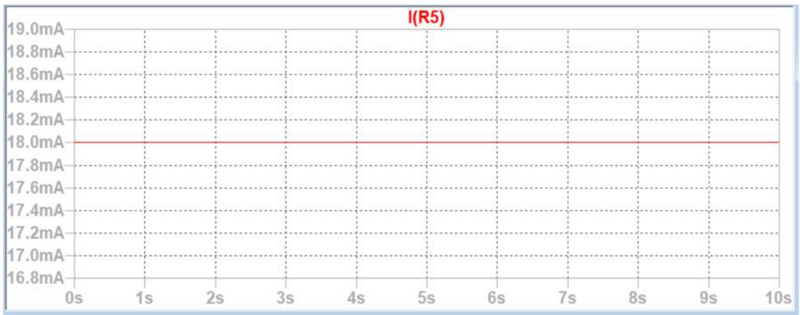
Fig. 5.116: Circuit for question 2 (Current through the resistance R5 of the circuit shown in Fig. 5.114)
