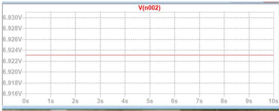
Fig. 5.112: Circuit for question 1 (Voltage at Point B of the circuit shown in Fig. 5.111)
