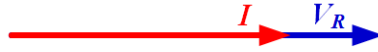
Fig.1.18 Voltage and current phasors of pure resistive circuit excited by sinusoidal ac voltage source
